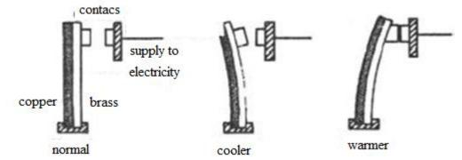
Based from the figure, if the bimetal was heated, it will....
