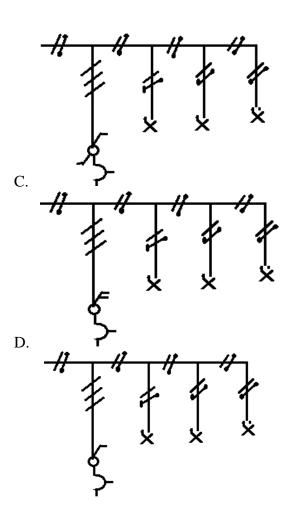
55. In the study room, there are two lamps that are turned on and turned off with a series switch, and an outlet. Outletis not depended on the switch. Wiring diagram to be made is ....
