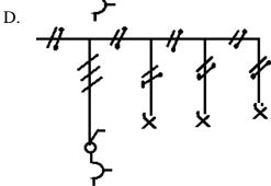
55. In the study room, there are two lamps that are turned on and turned off with a series switch, and an outlet. Outletis not depended on the switch. Wiring diagram to be made is ....
